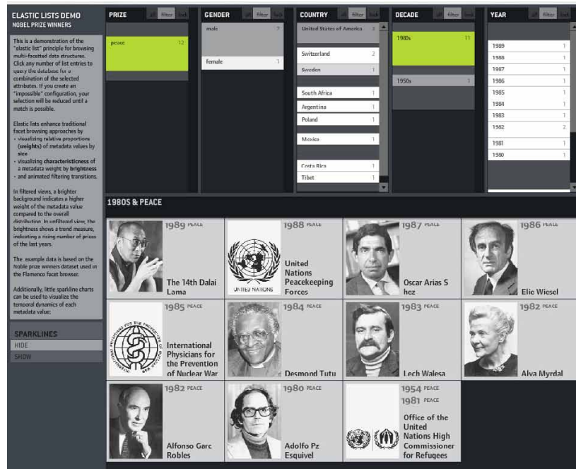
Figure 2.9: A screenshot of a demonstration of the elastic lists concept by Stefaner [60] in a faceted browser. Here the data source are Nobel Prize winners—in the current state of the faceted browser, the set is filtered by Peace prize winner from the 1980s. The height of each item in the facet-list encodes the number of appearances. The lightness indicates the unusualness of this facet value in the current context compared to the unfiltered set of results.
